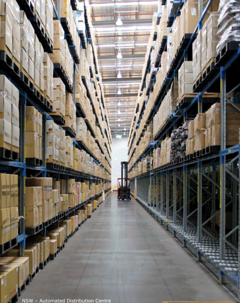
NSW – Automated Distribution Centre Three Tier Pick Modules, Pallet Racking, CLS, PLS, Pick to Light, and Conveyors
